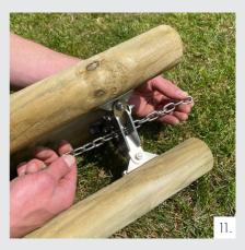
Pull half the chain through the hole and place it over the tube. Lock the chain between the tabs. See photo 12
