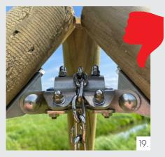
6. If a relatively heavy object is hanging on the hook, it may be more difficult to adjust its height. In this case, lift the hook with one hand and tension and lock the chain with the other. Do not hang too far forward above the fire!
