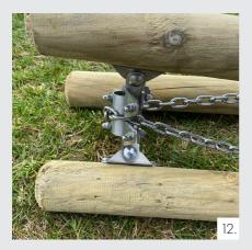
Place both ends of the chain parallel to the posts. The tripod can now be put upright. Make sure that the poles remain parallel to each other! Also keep the chain against the posts so that it does not swing around uncontrollably. See photo 13
