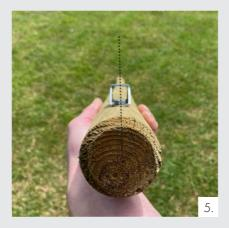
When the hinge is aligned, the second hole can be pre-drilled. Again 40mm deep and straight at the heart of the wood. Repeat this for all 3 posts.
